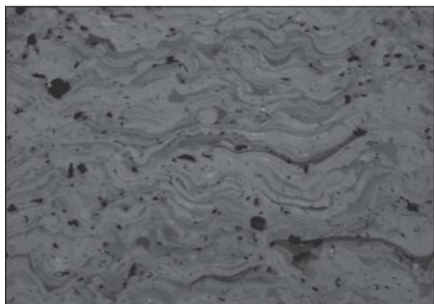
Fig. 9 Optical micrograph of APS TiO 2 coating
